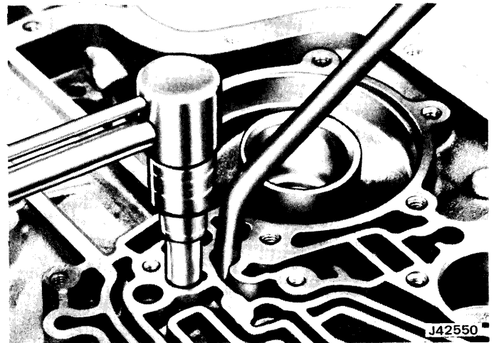
Fig. 7-132 Installing Center Support Bolt
