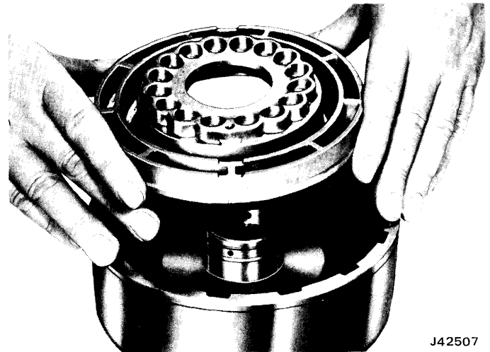
Fig. 7-82 Removing Piston from Direct Clutch Housing
