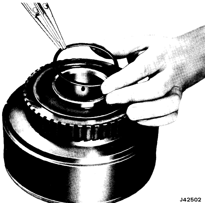
Fig. 7-77 Checking Forward Clutch Operation
